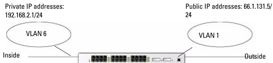
Figure 3 Example: Source NAT using Controller IP Address
